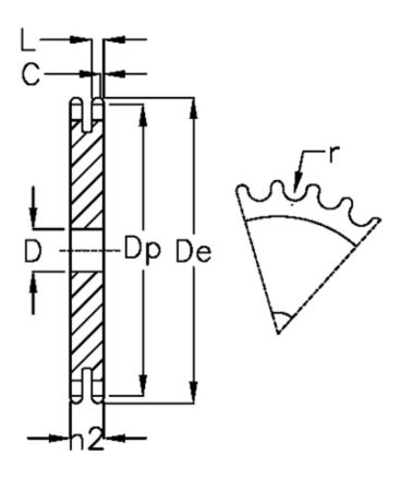
C = 2 D = 30 De = 385.1 Dp = 376.12 For chain size =  $3/4 \times 7/16$ For chain type = 12 B-2 h2 = 30.3
